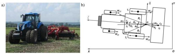
Fig. 1. Agricultural tillage unit New Holland T 8. 390 + DHM-8.0 (modernized disc harrow): a – general view of the unit; b – design scheme
